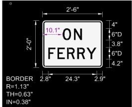
This sign will be installed 1.0" below the R14-5 sign. Sign is modeled after a W16-3P, but with different coloring. 30.00" x 24.00"
