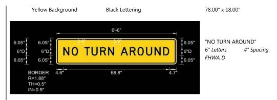
These two signs will be installed on one assembly with the yellow sign mounted 1.0" below the white sign. Assembly shall be installed on Type D slip bases, set in concrete, per KYTC Standard Drawings.
