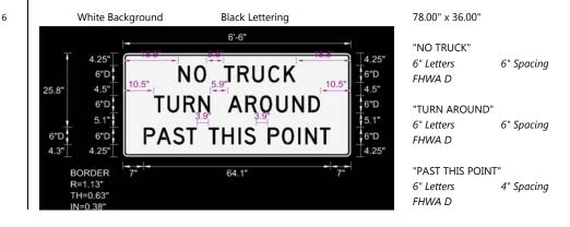
On two posts, with bracing, per KYTC Standard Drawings
