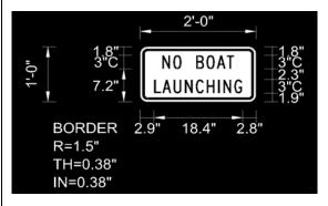
The "NO BOAT LAUNCHING" sign will be installed 1.0" below the "BOAT LAUNCHING PROHIBITED SYMBOL" sign.
