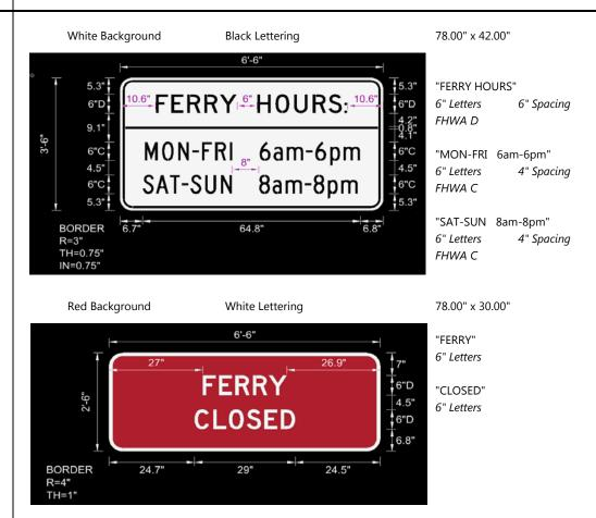
"Ferry Closed" sign should be manufactured in two 15" height segments.
